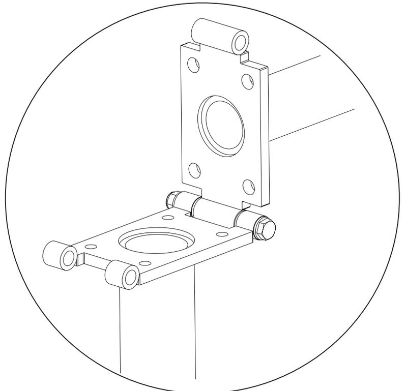
**ADDITIONAL MAINTENANCE:** For smoother operation and to prevent rust periodically grease hinge.
