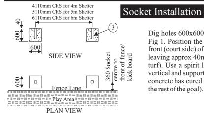
Dig holes 600x600 square x 600mm deep at centres shown in Fig 1. Position the sockets (3) 360mm centrally back from the front (court side) of the fence/kick board. Concrete the sockets in leaving approx 40mm from top of concrete to ground level (for turf). Use a spirit level to make sure that the sockets are truly vertical and support until set. Replace the turf extracted when the concrete has cured (allow the concrete to set before assembling the rest of the goal).
