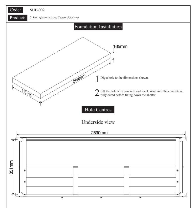
Place the Shelter in position and mark out the hole centres through the fixing lugs in the Sideframes.
