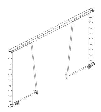
Once the goal has been folded the wheels will drop into position, allowing the goal to be easily moved.
