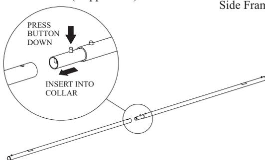
Insert Back Bar into Side Frame Collar
