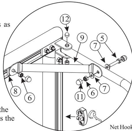
The Back Bar should now be inserted into the collar on the back of each side frame. Depress the button clip to engage into the hole in the collar.
