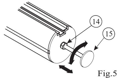
**IMPORTANT NOTE:** If elbow brackets are to be used, please consult INS557 (Aluminium Elbow Football Bracket Instructions) before proceeding as an additional square head bolt needs to be fitted. If intending to fit a hinged bottom net support, see INS529 as the back plate should be inserted before the crossbar is fitted.
